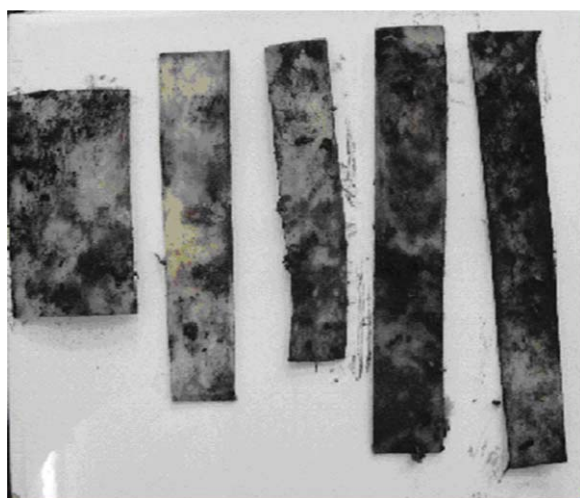
Figure 15. Images of Aspergillus niger growth on PU/GS green composites. [Color figure can be viewed in the online issue, which is available at wileyonlinelibrary.com.]
